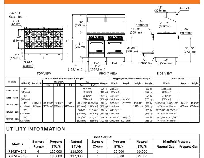
R482ST – 48B 256,000 2 54,000 4" W.C 10" W.C 8 240,000 60,000 60,000 R602ST - 60B 320,000 10 300,000 2 65,000 R722ST - 72B 12 360,000 384,000 2 66,000 70,000 \*NOTE: Models R482ST-48B and R602ST-60B come with a standard oven and a space saver oven standard. Space saver oven 27,000 BTU/h (LP)
